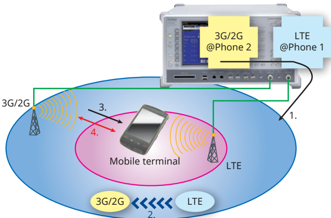
Connection Example with the MT8820C: MT8820C × 1 unit (supports parallel-phone measurements)
